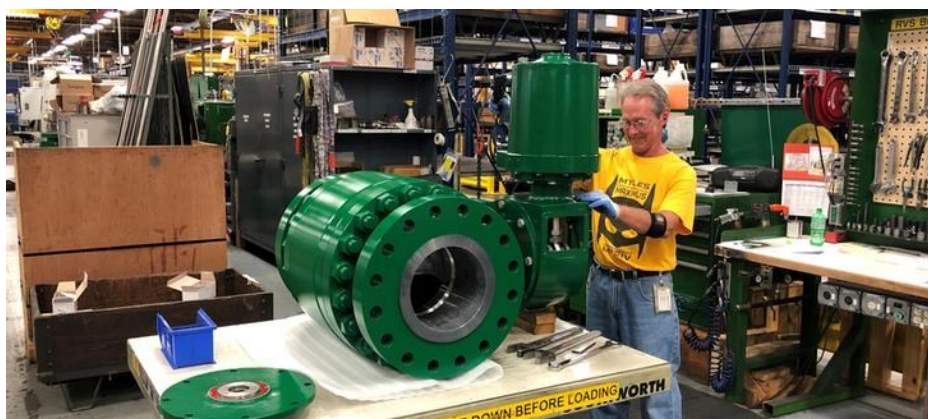
A file photo of a worker assembling an industrial valve at Emerson Electric Co.'s factory in Marshalltown, Iowa, U.S., July 26, 2018. REUTERS/Timothy Appel
